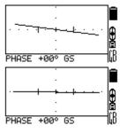
the searchcoil (a clod or an air layer) and during scanning these pieces go one after another, sometimes it leads to phantom responses of the device identification channel. At the same time, ground phase digit in automatic balancing operation may differ by 3 degrees on the same place.
