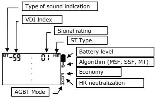
VDI means Visual Discrimination Indication. VDI Index This is a so-called electrical conductivity indication of the object.
